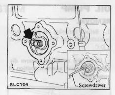
4. Smear a little engine oil on rubber gasket of oil filter.
