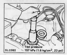
If the pressure drops, check for leaks from hoses, radiator, or water pump.
