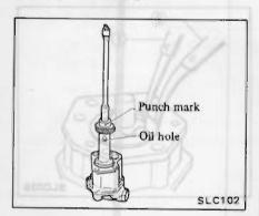
3. Using a new gasket, install oil pump and drive spindle assembly.
