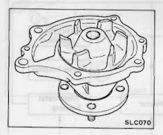
Inspect water pump bearing. Check for excessive end play or rough operation.
