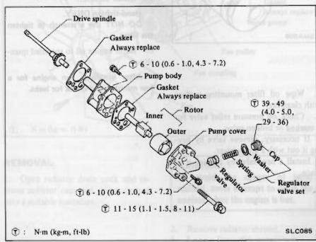
2. Check oil pressure regulator valve sliding surface and valve spring.
