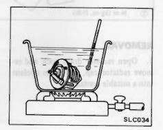
3. Then check if valve closes at 5°C (9°F) below valve opening temperature.
