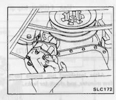
The dot on outer and inner rotor should face toward oil pump body.
